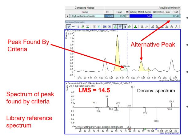
Quant method criteria chooses the primary peak based on target qualifier ratio and RT
